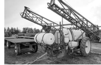
Hardi HC950M , S/A sprayer, PTO pump, 12x38 tires, 75' hyd. booms, triple nozzles, 20" spacing, #44724, $9,500.
