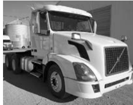
'14 Volvo VNL, D13 Volvo, 405 hp, 12 spd., auto., PS, A/C, Jake, air ride, 12F, 40R, 180" WB, $49,500.
