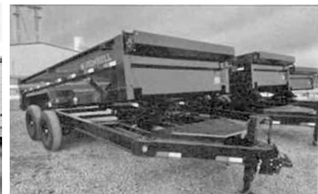
'22 Ironbull 7'x14' 14K dump , 8" I-beam frame & tongue, 4" tubing bed frame, 7-ga. floor, 24" 10-gauge steel sides, oversized frt. toolbox, 10K drop leg bolt-on jack, 3-way rear gate, retractable tarp system, std. slide-in ramps, super lube hubs, 5-amp 12-volt wall charger, $11,925.
