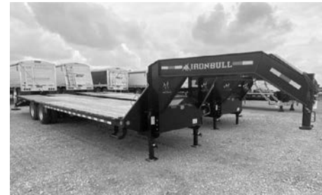
'22 Iron Bull 8.5'x27'+5' gooseneck deckover trlr. , 27'+5"x102", 22,000 GVW, (2) 10,000 lb. axles w/easy lube hubs, 16" radial tires on steel whls. (235/80R16) 10-ply, (2) 10000 lb. drop leg jack, 5' self-cleaning dovetail w/ Rampage ramps, all LED lights, treated pint 2"x6" floor, (8) weld in D-rings, frt. full size tool box $20,300.
