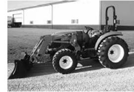
MT352, 2700# ldr. lift cap., joystick, 2-factory rear rem., telescopic 3-pt. hitch, skid steer style quick attach.
