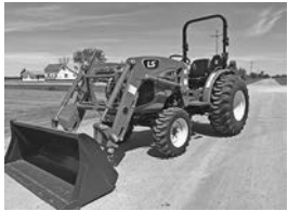
MT240HE, MFWD, hydro, 40 hp, quick attach ldr. & bucket incl., foldable ROPS, shuttle, 3-pt., PTO, joystick, backhoe avail. separately.
