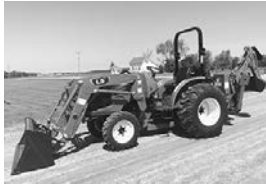
MT235EH w/LB1100 backhoe & LL3301 ldr., installed, MFWD, joystick, 2-rem., 28 hp, PTO, 113" neck.
