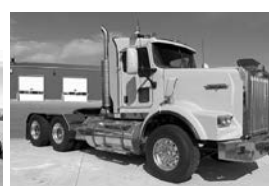
'07 KW T800 , yellow, C15 475 Acert, 450,000 miles, 18,000 hrs., 18 spd., 46-170HP rear, 4.30 ratio, drum brakes, 180" WB, wet kit, new frame paint, $89,900.
