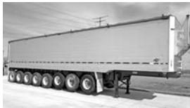
'17 Titan 8-axle dump , alum box, man door, grain chute, side-to-side tarp, drum brakes, 102" wide, 86" sides $115,000.
