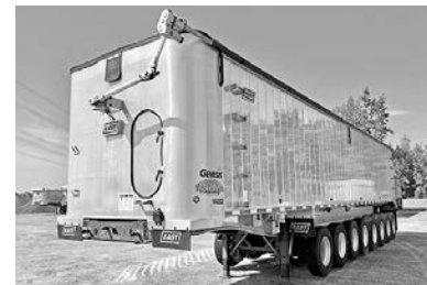
'14 East 8-axle dump, 42' long, drum brakes, alum. frame, man door, grain door, 11R22.5 tires, side to side elec. tarp w/rem., 102" wide x82" side, $135,000.
