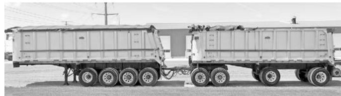
'02 Benson super trains, liners, tarps, alum. whls., hub pilot, Reyco 21B susp., 96"x66" sides, $79,900.
