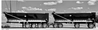
NEW '26 MAC super train , high liftgates, spg. ride, drum brake, 96" wide, 66" tall sides, AR450, call for more info.
