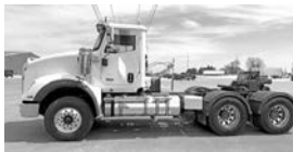
'17 Int'l. HX620 , Cum. ISX15, 600 hp, 263,000 miles, 12,590 hrs., drum brakes, lockers, 180" WB, wet kit, 3.91 ratio, 46R, RTLO(F)-18918B, 18 spd., $79,500 or best offer.
