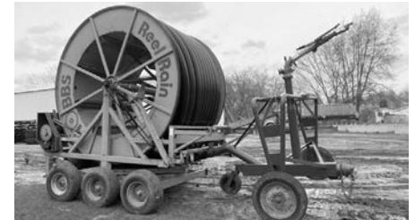
Hobbs RR3450 , Reel Rain irrigation hose wagon, 1/4 mile of 5" hose, high pressure water gun, #40686, $10,500. (N)
