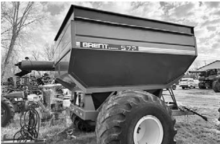
'93 Brent 572 grain cart w/scales, 66x43-25NHS Goodyear tires, 570-bu., S/A, scale, $11,500.
