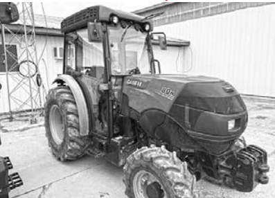
MY17 Case IH Farmall 80N, 1243 hrs., MFD, Deluxe cloth air seat, 540/1000 PTO, 2-rem., 16x16 synchro, 16.9 gpm, 80 hp, $33,950.
