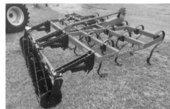
New Unverferth Perfecta 12, 3-pt., 8' working width, spike bar, rolling basket harrow, heavy S-tines, $5,150.
