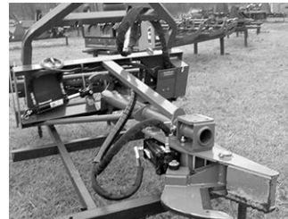
Tree shear for your compact tractor or skid steer, 8" universal mount, manual extension, 359° rotation.
