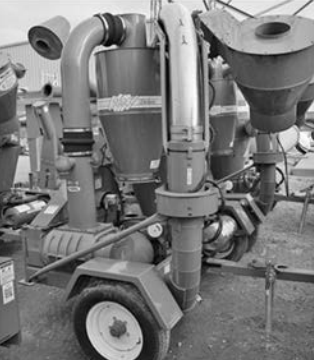
'09 Walinga Agri-Vac 7614 DLX, orig. airlock & paint, secondary dust collector, hyd. boom lift & rotation, 5000-bu./hr. cap., $27,000.
