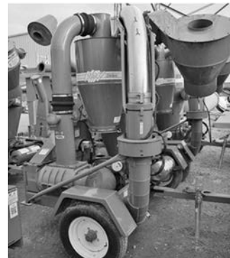
'09 Walinga Agri-Vac 7614 DLX , orig. airlock & paint, secondary dust collector, hyd. boom lift & rotation, 5000-bu./hr. cap., #11801, $27,000.
