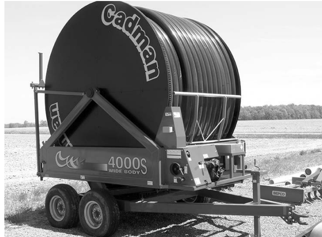
Cadman 4000SWB Traveler, tdm. axle, 4"x1250' PE tube, Komet 160 Big Gun, turntable, 5.5 Honda eng. drive.
