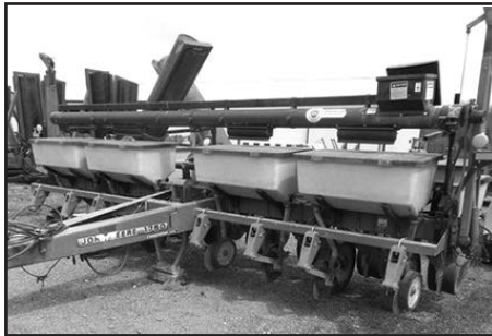
(S) 1997 JD 1750, 8 ROW 30" PLANTER, VAC. DRY FERT., WITH FILL SYSTEM, SINGLE DISK OPENERS, 150 MONITOR, SEED HOPPER EXTENSIONS, D/P SPRINGS, CORN AND SOY-BEAN PLATES, #93184, $18,500.
