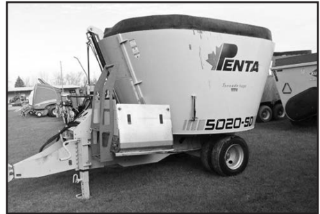
(BA) 2012 PENTA 5020-SD, SINGLE AUGER VERTICLE MIXER, WITH FRONT DOOR AND CONVEYOR TO THE RIGHT SIDE WITH INCLINE, DUAL TIRES, 2 SPEED GEAR BOX, DIGISTAR EZ2500 SCALE, #92059, $21,000.
