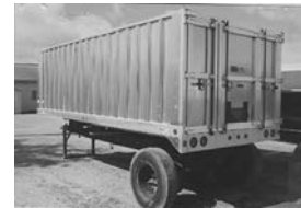
New all alum. Dakota 19"x96", 62" sides, ladder bolt on side of box over tires, 3/16 alum.extruded inner locking floor, C/M 4" channel on 15" centers, long beams 8" alum. channel, top rail 4x4x3/16 tubing, 3-pc. swg. tailgate, w/H.D. hinges, (3) latches, grain hole, $13,090 plus taxes & freight, your choice of hoist.
