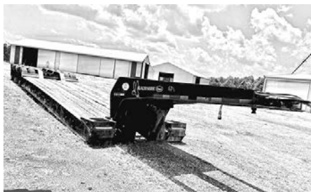
'98 Blackhawk Etnyre RGN lowboy trlr., air ride, 26' well, 102" wide, non-ground bearing, $26,000 or best offer .
