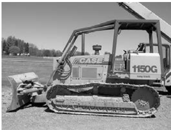
'99 Case 1150G dozer, OROPS, turbo, long track, 8'6" overall width, 22" pads, 110"x42" blade, 26,300 lbs., 118 hp, $29,900.
