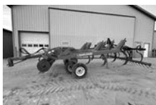
Sunflower 4212 7-shank disc chisel plow , S-tine & buster bar leveler, hyd. adj. discs, $15,900.
