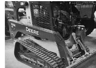
'16 JD 323E, 130 hrs., cab enclosure, A/C, EH controls, ride control, narrow rubber offset tracks, GP 72" bucket, sgl. spd., std. hyd., 2" seatbelt, pwr. quick tach, cab, heat, A/C, std. fan, horn, backup alarm, ctr. wt., AM/FM radio, 72" construction mech. seat.
