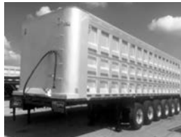
'00 Alfab 36'x102"x90" 6-axle, 120 liner, new paint on frame.
