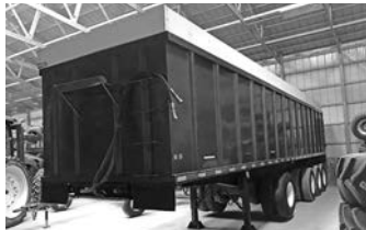
'80 Thumb, 34'x96" tri-axle, plus 9' spread.
