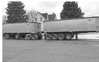
'11 East super trains, 72" sides, 102" width, bedliner, Shur-Lok roll tarp, air ride.
