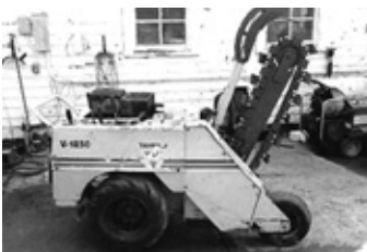
Vermeer V1850 trencher, 18 hp gas, hydro, 653 hrs., $2,750.
