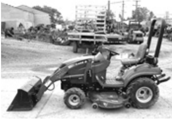
Case IH DX22E, 22 hp, 3-cyl. dsl., 4WD, 3-pt., hydro trans., ldr., 60" mid-mount mower, 234 hrs., very clean, $12,000.
