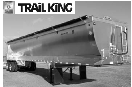
New Trail King alum. belt trlr., 43'x102", 63 cu. yd., floor & wall liner, LED lights, 11R22.5 General ST250 14-ply tires, all alum. whls., 48" belt w/sgl. drive conveyor, reverse roll tarp w/8" rise flexbows, alum. grain chute, $79,000.
