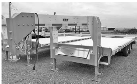
New '18 Eby gooseneck deck over equipment trlr., 24'6"x102'; alum., (2) 7000# axles, 15,900 GVW, elec. brakes, alum. whls., 51" beavertail, (2) 30" fold flat ramps, toolbox mounted between jack legs, (4) pocket mount D-rings, #64534, $14,650.
