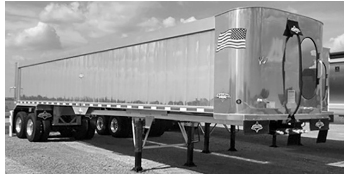
New '17 Trailstar dump trlr., 39'x96"x60", alum. smooth side polished frameless type dump trlr., CM's 12" apart, LED lights, driver side bulkhead man-door, 1st panel ladders in, rear panel in & out ladders, shovel hanger, 14" alum. handle locking coal door, air ride, 11R22.5 tires, all alum. whls., stand. & full across rear mudflaps, custom 8-5-265 hoist, alum. 224" draft arm, $54,500.
