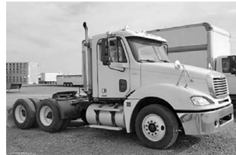
'07 FTL CL12064S semi truck, white, Det. 60 Series, Fuller 10 spd. manual, eng. brake, air ride susp., 455 hp, 295/75R22.5 tires, all steel whls., 3.55 ratio, 165" WB, 52,000# GVW, air ride cab, dual 80-gal. alum. fuel tanks, sldg. 5th whl., tilt/tele., cruise, susp. dump valve, 551,800 miles, $31,900.
