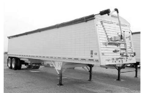
Used '14 Wilson hopper trlr., 42'x96"x72", alum. trlr., white, 11R24.5 tires, (4) alum. & steel whls., air ride, S.S. rear & frt., ag hoppers, strap trap doors, (1) row of (5) LED lights, elec. tarp, upper & lower knock rails, #64594, $28,500.
