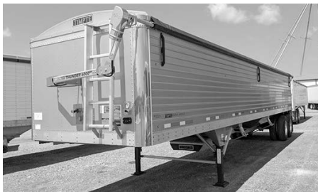
New '19 Timpte 40'x96"x66" hopper trlr., silver frt. & walls, S.S. frt. corners & rear, (2) rows of (5) clear bullet lights, (7) clear bullet lights on rear header, air ride, ag hoppers, sgl. spd. openers, 11R22.5 tires, (4) alum. & (4) steel whls., 18 oz. black tarp, Thunderstone elec. tarp, $40,900.
