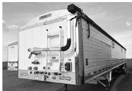
Used '14 Wilson hopper trlr., 40'x96"x66", alum. trlr., white, 11R24.5 tires, (4) alum. & steel whls., spg. ride, good tarp, split tub, (1) row of (5) LED lights, S.S. frt. corners, Shurco elec. tarp & traps, #64801, $25,500.
