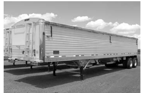
'15 TimpTE trlr., 40'x96"x66", alum., white, air ride, ag hoppers, all alum. whls., 11R22.5 tires, S.S. frt. corners, frt. splash guards, (2) rows of (3) LED lights, permit holder, $29,900.
