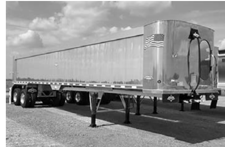
'17 Trailstar dump trlr., 39'x96"x60", alum. smooth side polished frameless type dump trlr., CM's 12" apart, LED lights, driver side bulkhead man-door, 1st panel ladders in, rear panel in & out ladders, shovel hanger, 14" alum. handle locking coal door, air ride, 11R22.5 tires, all alum. whls., stand. & full across rear mudflaps, custom 8-5-265 hoist, alum. 224" draft arm, $54,500.
