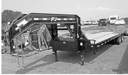
PJ FD flatdeck , model GNFD208530, 12" frame, 25,000 GVW, 30'x102", 5' dovetail, Monster ramps, LP cold harness, 2 spd. jack, $11,400.
