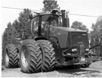
'10 Case IH 385 Steiger, 5325 hrs., bare-back, full auto. steer, (2) beacons, htd. seat, diff. locks, elec. mirrors, 620/70R42 @ 85%, 4-rem., full wt. pkg., w/'11 Grouser, 14' model 450 Ag Pro blade, pkg. $116,000, call for separate price.
