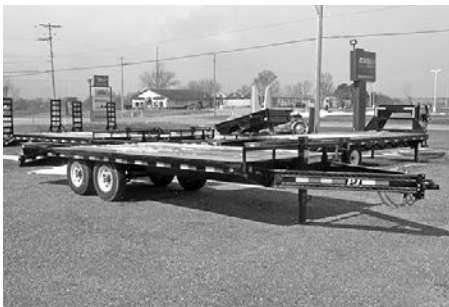
PJ trailer , deckover, 14,000 GVW, 8'x20', 4' dove w/(2) ramps, $5,150.
