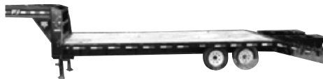
8-1/2'x25' Gooseneck, tool box, 14,000 GVW, 5' dovetail, (2) flip ramps, powder coat paint, sealed wire harness, $6,190.
