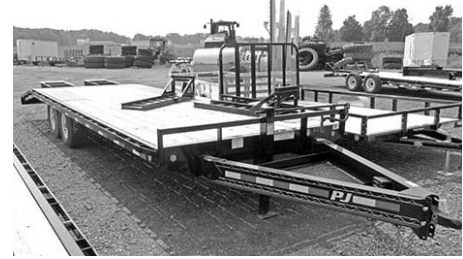
PJ F8 deckover , model BPDO148024, 8" frame, 14,000 GVW, 24'x96", 3' dovetail, 2 ramps, cold harness, pintle, $5,755.
