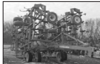
'99 Brillion HFCT45 field cult., w/ Remlinger 3-bar spike, roller, rear hitch & hyds.
