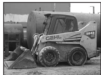
'11 Gehl 5640E skid ldr., cab, A/C, heat, T-bar, 2 spd., pwr. A-tach, 12x16.5, 74" bucket, 3026 hrs.
