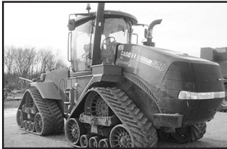
'13 Case IH 500QT, 30" tracks, diff. locks, HC pump, HC draw bar, 6-rem., semi-active seat, instruct. seat, HID light pkg., hyd. ret., radar, 970 hrs.
