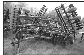
'03 Case IH MRX690 7-shank mulch till ripper, 7" points, coverboards, spg. reset, hyd. disc gangs, hyd. wing fold.
