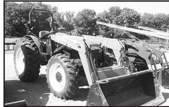
'09 NH TT75A, MFD, ROPS, 11.2x24, 16.9x30, 3-pt., 540, 1-rem., 620TL ldr., 72" bucket, 1210 hrs.
