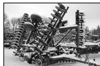
'12 Case IH 340 31' Tru tdm. disc., cushion gang, 22" 6.5 mm blades, hyd hitch, opt. gang brgs., 3-bar coil tine.
