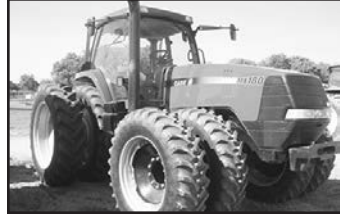
'01 Case IH MX180 Magnum, C-A-H, 380/85R34 duals, 480/80R46 duals, 3-pt., QC, 540/1000 PTO, 3-rem., hyd. ret., instructor seat, wt. bracket, 6622 hrs.
