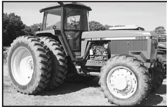
JD 4960, MFD, C-A-H, 380/85R38, 18.4x46 duals, 3-pt., QH, 1000 PTO, 3-rem., (16) ft. wts., (2) 150# whl. wts., PS trans., 7395 hrs.
