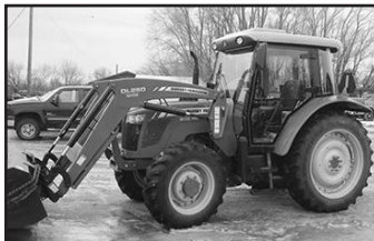
'10 MF 2660 HD, cab, A/C, heat, AWD, 12.4x24, 15.5x38, 3-pt., 540 PTO, 2-rem., 8x8 C/S, DL260 ldr., 84" Q.A. bucket, 1105 hrs.
