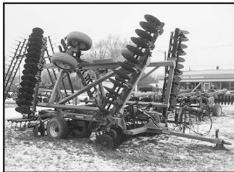
'12 Case IH 340 31' disc, HD gang brgs., 22"x6.5, MM blades, hyd. hitch leveling 3-bar coil tine.
