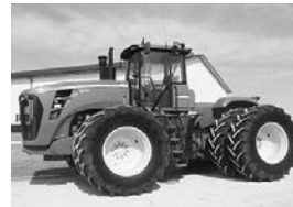
'08 JD 9430, 710x38 rubber, 10-bolt duals, ins. whl. wts., 4-hyds., pwr. shift, bareback, 1 hr. on rbit eng., new injectors, new oil cooler, water pump, all new valves, new balancer, $100,000.
