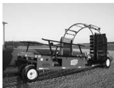
262PR02 Kemco bale wrapper, 4-film disp., 20 hp Honda, dual whl. drive, wraps up to 6'6" round bales & 7' square bales, $29,750.
