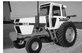
'79 Case 2090, 18.4x38, 2-hyd., 540/1000 PTO, diff. lock, cold A/C, recent new paint, one-owner, frt. wts., $14,500.
