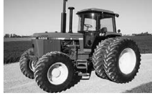
'84 JD 4450, MFWD, 20.8x38 rubber, 10-bolt hubs & duals, frt. fenders, PS, 2-hyd., 3-pt., 540/1000 PTO, new paint, $34,500.
