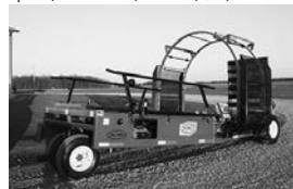
262PRO2 Kemco bale wrapper, 4-film disp., 20 hp Honda, dual whl. drive, wraps up to 6'6" round bales & 7' square bales, $29,750.
