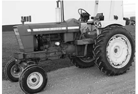
'89 JD 4255, 18.4x38 rubber, 2-hyd., 540/1000 PTO, quad, new paint, $30,500.
