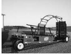
262PR02 Kemco bale wrapper, 4-film disp., 20 hp Honda, dual whl. drive, wraps up to 6'6" round bales & 7' square bales, $28,750.
