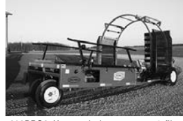
262PR02 Kemco bale wrapper, 4-film disp., 20 hp Honda, dual whl. drive, wraps up to 6'6" round bales & 7' square bales, $29,750.
