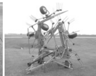
Kuhn 7802, 6-spindle tedder.
