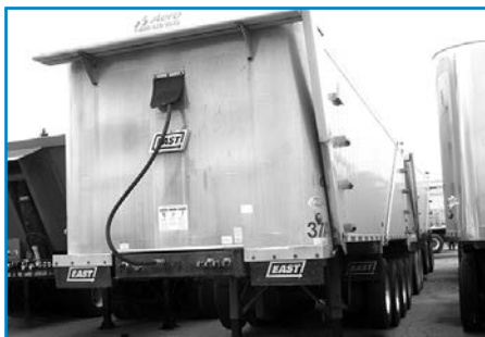
'11 East super trains, alum., mouse trap tarps, liner, 72" sides, 102" wide.
