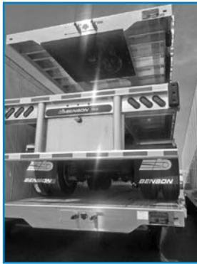
'17 Benson 48'x102" alum. flats, spread axle, alum. floor w/(3) Apitong wood nailers, 16" CM's, (12) sldg. winches.
