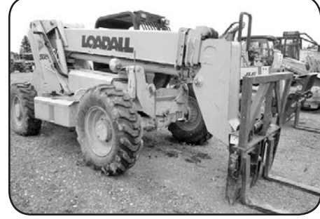
'99 JCB 508C telescoping forklift, ROPS, 4x4, 2-whl., 4-whl., crab steer, 8000 lbs. lift cap., 42' reach, 13x24 tires, rear foam filled tires, QT fork carriage, 48" tines, aux. hyd., body lean, 4-cyl. Perkins dsl., tilt on the forks, 3630 hrs., weighs 25,000 lbs., runs & operates good, $29,500.
