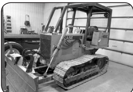
'85 Case 450C dozer, ROPS/Sweeps, 88" wide, 6-way blade, 18" pads, drawbar, 4-cyl. Cum., dsl., high/low trans., 5-roller btm., 63 hp, weighs 12,500 lbs., 4558 hrs., runs & operates great, $14,500.
