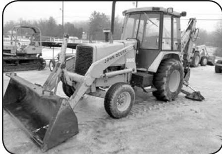
'87 JD 310C backhoe, cab, heat, 2WD, E-hoe, 18" rear bucket, 90" frt. bucket, 19.5-24 rear tires, 11Lx16 frt. tires, 2 lever controls, shuttle trans., 4-cyl. JD dsl., 65 hp, eng. block heater, weighs 13,000 lbs., 6078 hrs., runs & operates great, $12,900.
