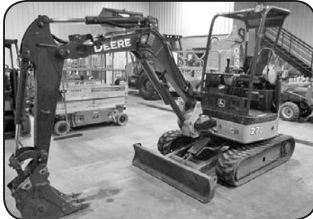
'12 JD 27D mini excavator, ROPS, 12" rubber tracks, 61" wide blade, 12" QT bucket, 47" stick aux. hyd., pattern changer, 2 spd. travel, 3-cyl. Yanmar dsl., boom swing, weighs 6400 lbs., 27 hp, 1941 hrs., max digging depth 8'6" deep, runs great, nice excavator, $23,500.
