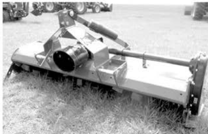
BUSH HOG TILLER RT84G 84", working width 82.5", 6 blades per flange, gear drivetrain, PTO w/slip clutch. $2,599
