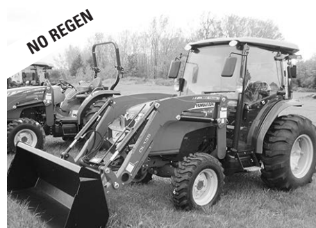
New MF 1755M , 55 hp, 4WD, 3-range hydro, 540 I-PTO, 1-hyd., MF DL135 ldr., joystick, skid steer QA, 72" bucket.
