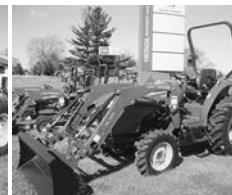
(2) New MF 1742 , 4WD, 42 hp, 12x12 pwr. shuttle, 540 ind. PTO, DL125 Idr.
