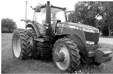
'13 MF 8670, 320 hp CVT, 480/80R50 rear, 380/80R38 rear duals, 4-rem., pwr. beyond, cab susp., 661 hrs., super deal $155,000.
