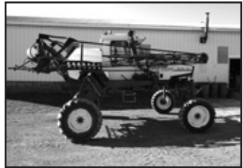
'96 Spra Coupe 3660, 3300 hrs., completely rblt. Cum. 3.3L, 4-cyl. eng., w/warranty, Raven rate controller, 60' booms, foamer, 120" row spacing, man. trans., frt. 11.2x24 lug style 90%, rear 13.6x24 lug style 60%. . . . . $28,900
