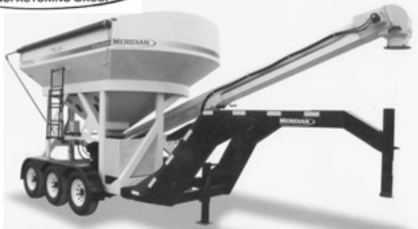
New Meridian Seed Express tenders, self filling, telescoping arm, variable spd., rem. control, dual compt., Honda gas, elec. start.
