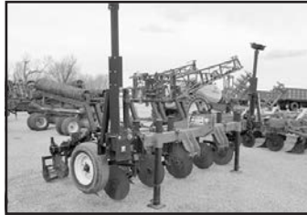
Unverferth Zone Builder 130 , 5-shank, 30" spacing, markers, disc closers, rolling baskets . . . . . $12,500
