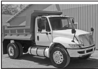
'13 Int'l. 4300 , DT466, 260 hp, 5.29 ratio, Allison RDS auto., 33,000 GVW, spg. susp., NEW 10' dump. . . . . $42,900
