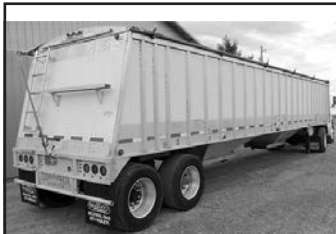
'08 Cornhusker 800 , 40'x72"x102" air ride susp., alum. whls., super singles, roll tarp, alum. frame, R.U. doors, (2) hoppers. .... $18,900
