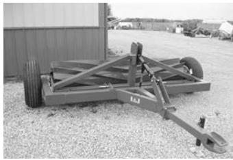
New I&J 8' cover crop roller , 3-pt. or skid steer mount, discounts on early 2019 orders, 8'-40' models.
