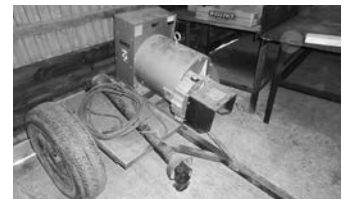
Winco 35,000 watt PTO generator, 540 rpm, w/trlr., $2,900.
