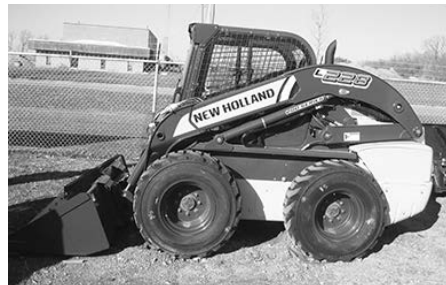
New NH L228 skid ldr. , 74 hp, 2800 lb. rated lift cap., cab, heat, A/C.
