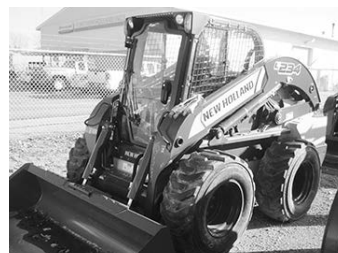
New NH L234 skid ldr., 90 hp, 3400 lb. rated lift cap., cab, heat, A/C.
