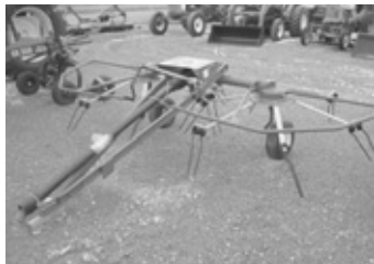
New Tonutti GT-310 hay tedder, 10'4" working width, $2,195.
