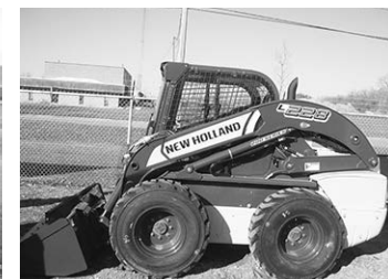
New NH L228 skid ldr., 74 hp, 2800 lb. rated lift cap., cab, heat, A/C.
