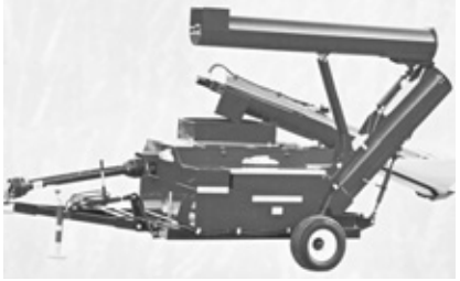
Auger discharge for minimal dust. Folds for easy transport.
