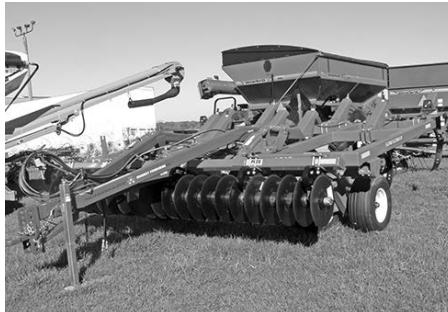
New Sunflower 4213 coulters chisel, 11-shank, hyd. adjust coulters, auto. reset shanks, call for pricing.
