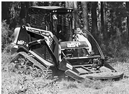
ASV RT30 compact track loader, 3,600 lbs. operating wt., 1,900 lbs. tipping load, 3.0 psi ground pressure, 32.7 hp gross eng. pwr.
