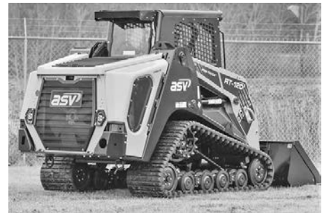
ASV RT120 compact track loader, 11,265 lbs. operating wt., 10,100 lbs. tipping load, 4.4 psi ground pressure, 120 hp gross eng. pwr.
