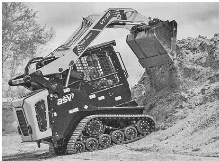
ASV VT70 compact track loader, 8,060 lbs. operating wt., 6,650 lbs. tipping load, 4.6 psi ground pressure, 65 hp gross eng. pwr.
