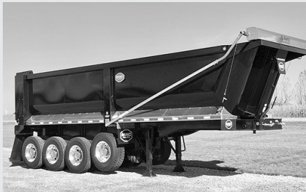
'18 MAC steel dump, black, rock tub, drum brakes, air lift gate, 1/4" thick box, optional tarp system shown. 28' Now in stock.
