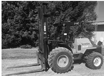
Master Craft Scrambler 4x4 8,000 lb cap rough terrain forklift, 14' mast, 5' forks, sideshift, see thru mast, Perkins diesel, 4300 hours . . $12,500
