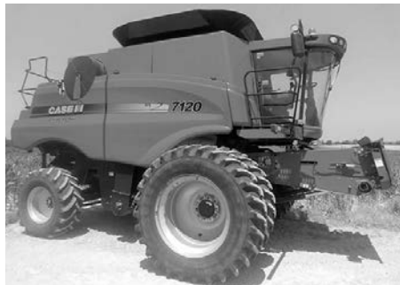
'10 CIH 7120, 1581E/1170S hrs., 2WD, 520R42 duals, full Auto Steer, PRO 600, 262 & NAV2 guidance, Rock Trap, field tracker, (2) HID & (3) beacon lights, 350-bu. grain tank, exc. rubber, super sharp!! $109,500.
