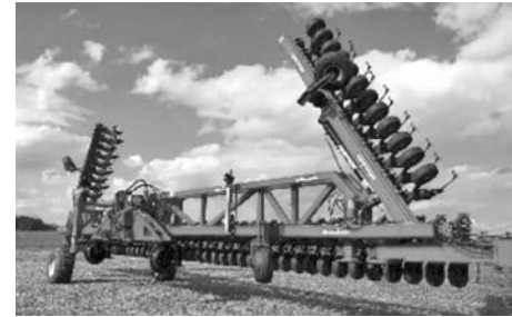
60' 3-pt. Mounted row cultivator available w/end transport.
