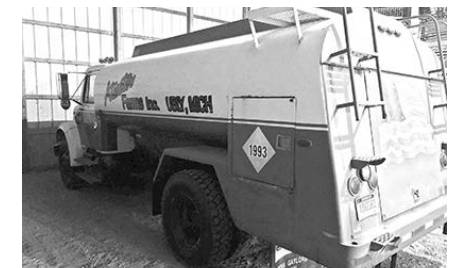
(2) Int'l. 4700, DT466, Allison auto., 4-compt. fuel truck, pump & meter w/long hose reel, $10,000 ea.
