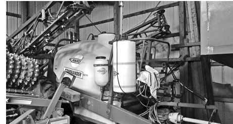
Hardi 750 Commander , foam markers, elect. controls, rinse system, chemical inductor, 60' HZ boom, Hardi diaphragm pump, consigned, 1-owner, $18,500.
