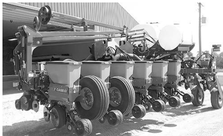
'12 Case IH 1250 , 16R vacuum planter, individual hoppers, pneumatic down pressure, liq. fert. w/ Sunco openers, 2x2 hyd. pump, starter fert. is in furrow w/totally tublar tubes, hyd. drive w/(2) section shut-offs, $49,500.
