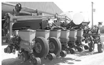
Case IH 1250, 16R vacuum planter, individual hoppers, pneumatic down pressure, liq. fert. w/Sunco openers, 2x2 hyd. pump, starter fert. is in furrow w/totally tubular tubes, hyd. drive w/(2) section shut-offs.
