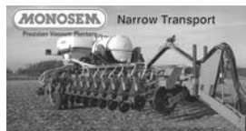
Transport width: 13'6" for single row, 17'6" for twin row. Pictured: 24R22" single row for beets in Michigan.
