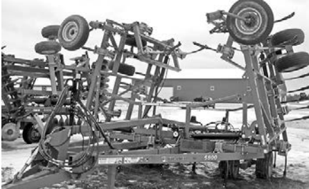
Wil-Rich 5830 37.5' chisel plow, OESS, 1000 compression spring, 15" spacing, castoring gauge whls., (4) 11Lx15 HD implement tires, 9.5Lx15 (8) pr. on wings, sgl. pt. hyd. depth control, $35,000.
