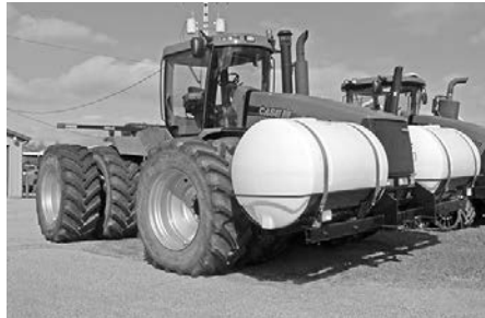
'09 Case IH Steiger 435, 710/70R42 Goodyear DT824 duals @ 90%, 4-rem., std. pump, diff. locks, std. drawbar, frt. wt. frame w/(8) wts., 5422 hrs., well maintained, $103,500.
