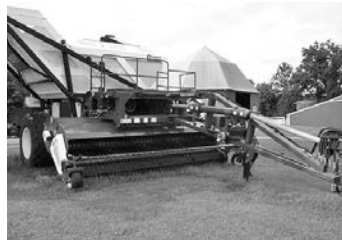
'14 Pickett Equipment Twin Master , edible bean combine, H.D. drive train, cam type cut-out clutch, over running clutch, 2.2 spd. trans. to threshing cyls., $180,000.
