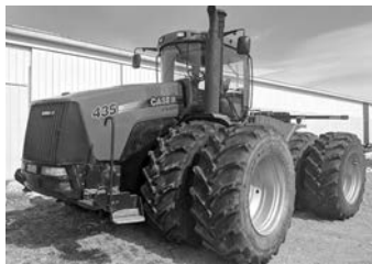
'09 Case IH Steiger 435 , 710/70R42 Goodyear DT824 duals @ 90%, 4-rem., std. pump, diff. locks, std. drawbar, frt. wt. frame w/8) wts., 5422 hrs., well maintained, $103,500.
