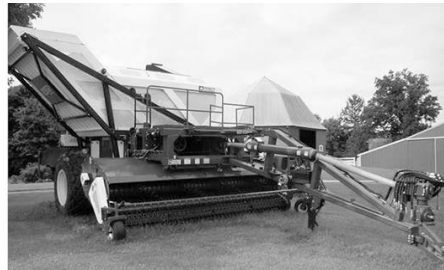
Twin Master edible bean combine standard features, H.D. drive train w/cam type cut-out clutch, over running clutch, 2.2 spd. trans. to threshing cyls., 1000 input, 540/390 output, optional trans. 500 & 350 output, in stock.
