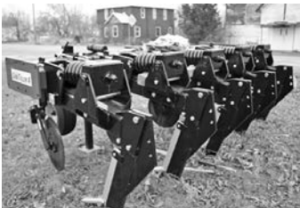
New Blu-Jet sub-tiller, rigid 11'3" base, auto. reset shank, 30" spacing, 20" blades, 3" points, call for price.
