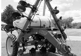
Blu-Jet 3015 liq. applicator, 32.5' toolbar, 13R30", 1025-gal. tank, Raven 450 rate controller, Ace 205 variable rate, hyd. pump, Orifice pkg., coulter knives, $31,500.
