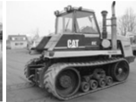
(2) '96 Cat CH85C, S/N 9TK- 01622, track drive, EROPS, heat & A/C, 4-rem., 35" rub- ber belts 30%, 3176 dsl., 370 hp, pwr. shift, Chevron drivers, 10 spd., avg. cond. $29,500
