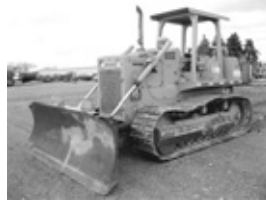
'98 Dresser TD12C XP, S/N 20753, OROPS, pwr. shift, 3 spd., lever steer, Cum. dsl., 24" pads, 95% U/C, 6-way blade, 1-owner ..... $39,500
